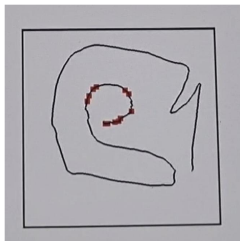
Figure 2 Enriched postponed condition. Red dots indicate abnormal velocity peaks on the trace, revealed after the trial. These peaks, identified using the SNvpd index (Danna et al., 2013), were computed by comparing velocity signals filtered at 10 Hz and 5 Hz (Butterworth low-pass filter). They correspond to areas where handwriting was less fluent.
